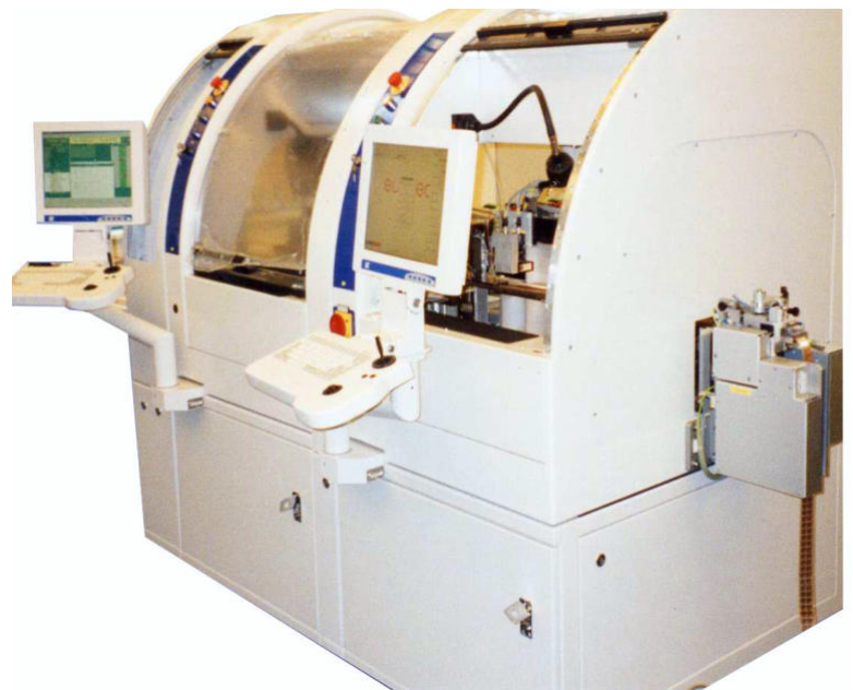
Semiconductor-series production IC multisite test with CT300 Meteor parallel test of 32 chips
