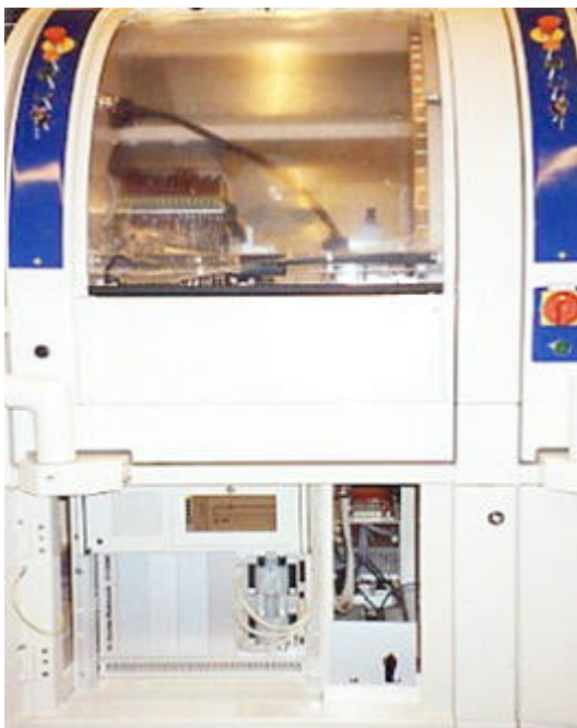
Semiconductor-series production IC multisite test with CT300 Meteor parallel test of 32 chips
