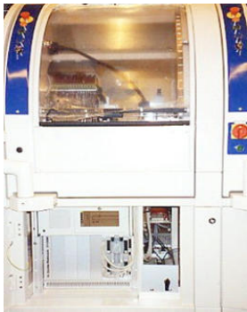
Semiconductor-series production IC multisite test with CT300 Meteor parallel test of 32 chips
